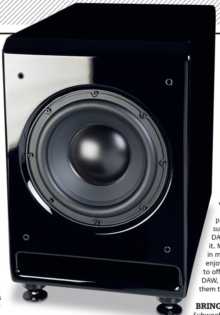
**LEFT:** A 250mm (10in) long-throw woofer is reflex-loaded via a front-firing slot port. The cabinet is supported and levelled using Wilson's heavy threaded spike and 'mechanical diode' arrangement
