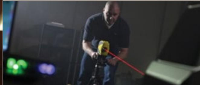
☞ Laser Vibrometry Analysis, long used in automotive and aerospace applications, allows us to measure mechanical vibrations in our cabinets down to the level of nanometers. This invaluable data allows Wilson to optimize the composite structure of the cabinet, as well as the position and thickness of the internal braces.
